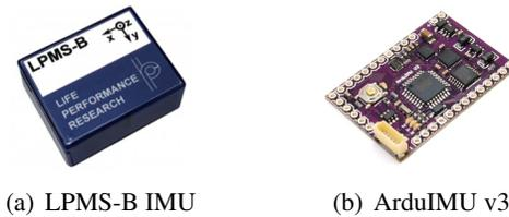
**Figure 10. Sensing devices considered in this research**
