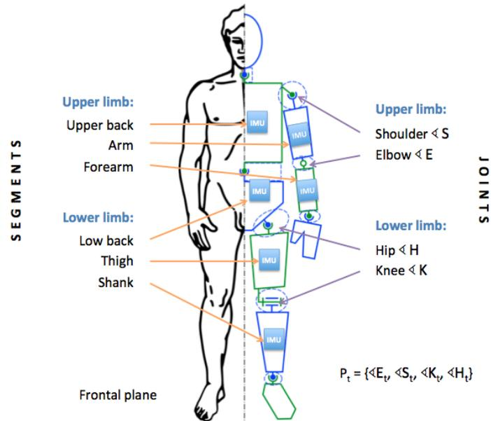
**Figure 13. Postures from a Wearable Inertial/Magnetic System**
