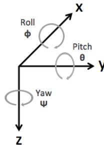
Figure 1. X, Y and Z coordinate system
