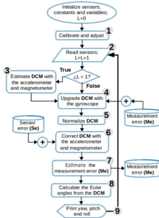
**Figure 16. Flow diagram used to calculate orientation, and then angles of pronation/supination and flexion/extension movements**
